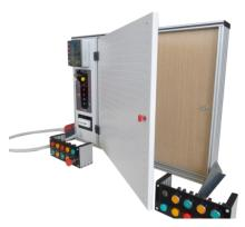
panels are hinged and can be opened, so students can have access to their back side. The 2 panels are separated by a wooden surface, 10 cm thick, installed in the frame, behind each of the perforated panels.
